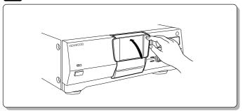
When a title name has been registered and the door panel is closed, reading operation is performed automatically.
